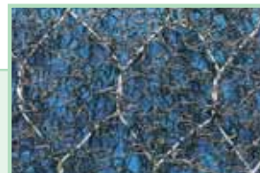
Slope and bank protection with geomats with geomats (Macmat® type) eventually reinforced during production with double twisted wire mesh or geogrids.
